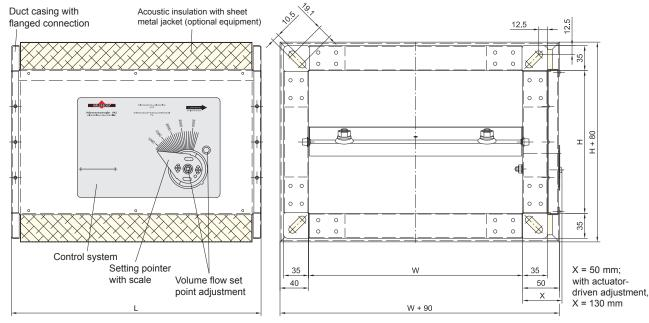
**VK2 volume flow controllers** are maintenance-free mechanical controllers that operate without an auxiliary power supply to maintain volume flows in ventilation and air conditioning systems constant.
