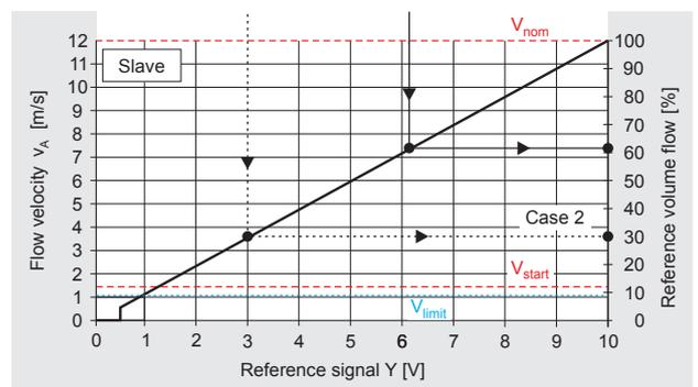
If the actual volume flow at the Master does not reach the reference volume flow, the Slave follows the actual volume flow!  $\Rightarrow$  see case 2
