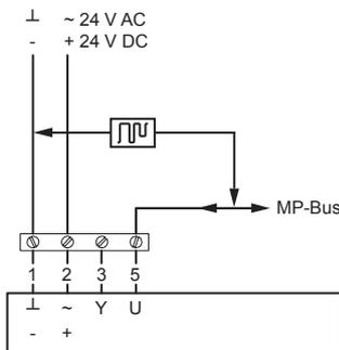
**Function:** The bus operation starts automatically once an address has been assigned. The actuator MP at the VRup volume flow controller represents one of a maximum of eight possible slaves (MP nodes), attached to an MP master. These receive their digital command signal from the MP master of the building control system (PLC or DDC controller with MP interface).
