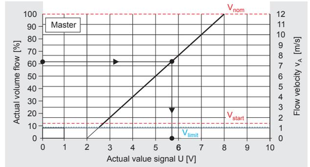
**Master** and **Slave** are set to 2 to 8 V in the "Variably adjustable" operation mode. The Master is set to  $V_{min} = 0\% V_{nom}$  and  $V_{max} = 70\% V_{nom}$  and controlled with  $Y = 2$  to  $8$  V.
