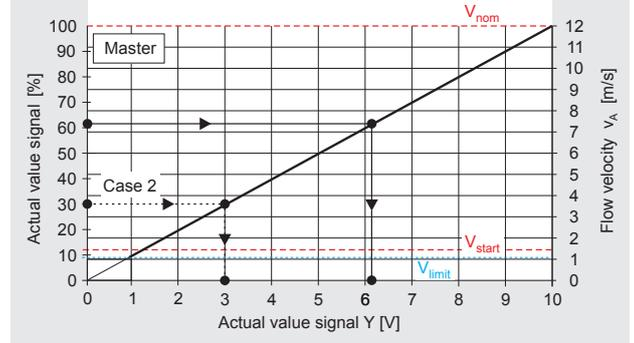
The operation modes "Variable 0 – 10 V" are set at the **Master** and **Slave**. The Master is then controlled with  $Y = 0$  to  $10$  V.
