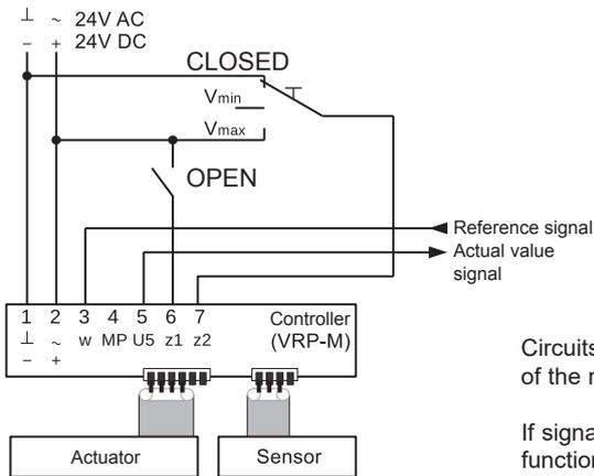
Circuits for override controls must be manufactured on site. Pay attention to mutual locking of the respective override controls (CLOSED,  $V_{min}$ ,  $V_{max}$ ) to avoid a short circuit!
