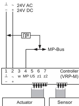
**Function:** The bus operation starts automatically once an address has been assigned. The VRP-M controller at the VRpro volume flow controller represents one of a maximum of eight possible slaves (MP nodes), connected to an MP master. These receive their digital command signal from the MP master of the building control system (PLC or DDC controller with MP interface).
