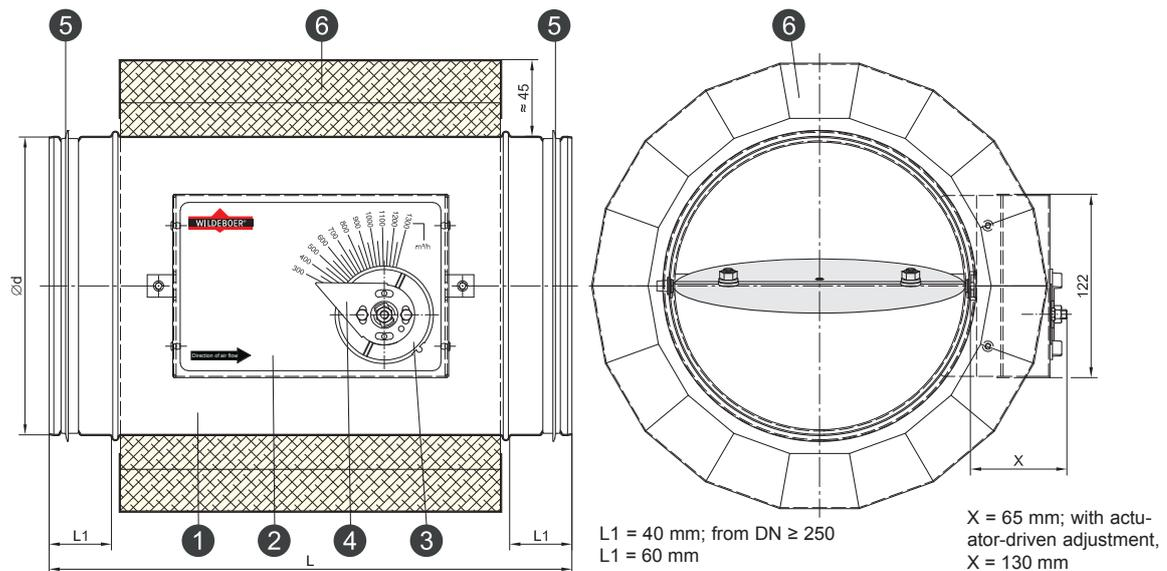
**VR1 volume flow controllers** are maintenance-free mechanical controllers that operate without an auxiliary power supply to maintain volume flows in ventilation and air conditioning systems constant.
