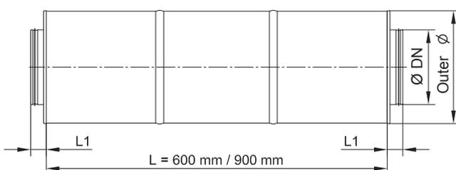
Maximum possible reduction of flow noise with sound attenuator lengths
